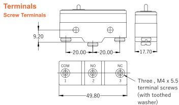
Appropriate terminal screw tightening torque: 0.78 to 1.18  $\mbox{N} \cdot \mbox{m}.$
